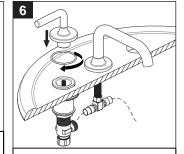
Place the "O"ring over the valve. Place the handle assembly on the valve. Secure the assembly by turning the handle hub clockwise.
