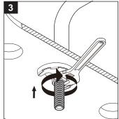
Carefully tighten spout nut to secure spout.
