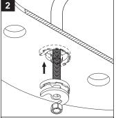
Slide "C" washer up on supply tube.
