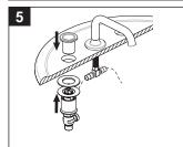
Push valve up from the bottom and thread on the valve sleeve from the top to secure the valve. If the deck is less than 1 3/8" thick use the supplied spacer. If the deck is thicker than 1 3/8" do not use the spacer.
