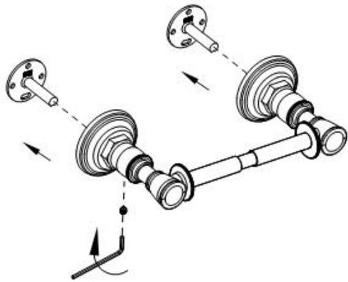
② ALIGN MOUNTING BRACKETS AND MARK LOCATION
