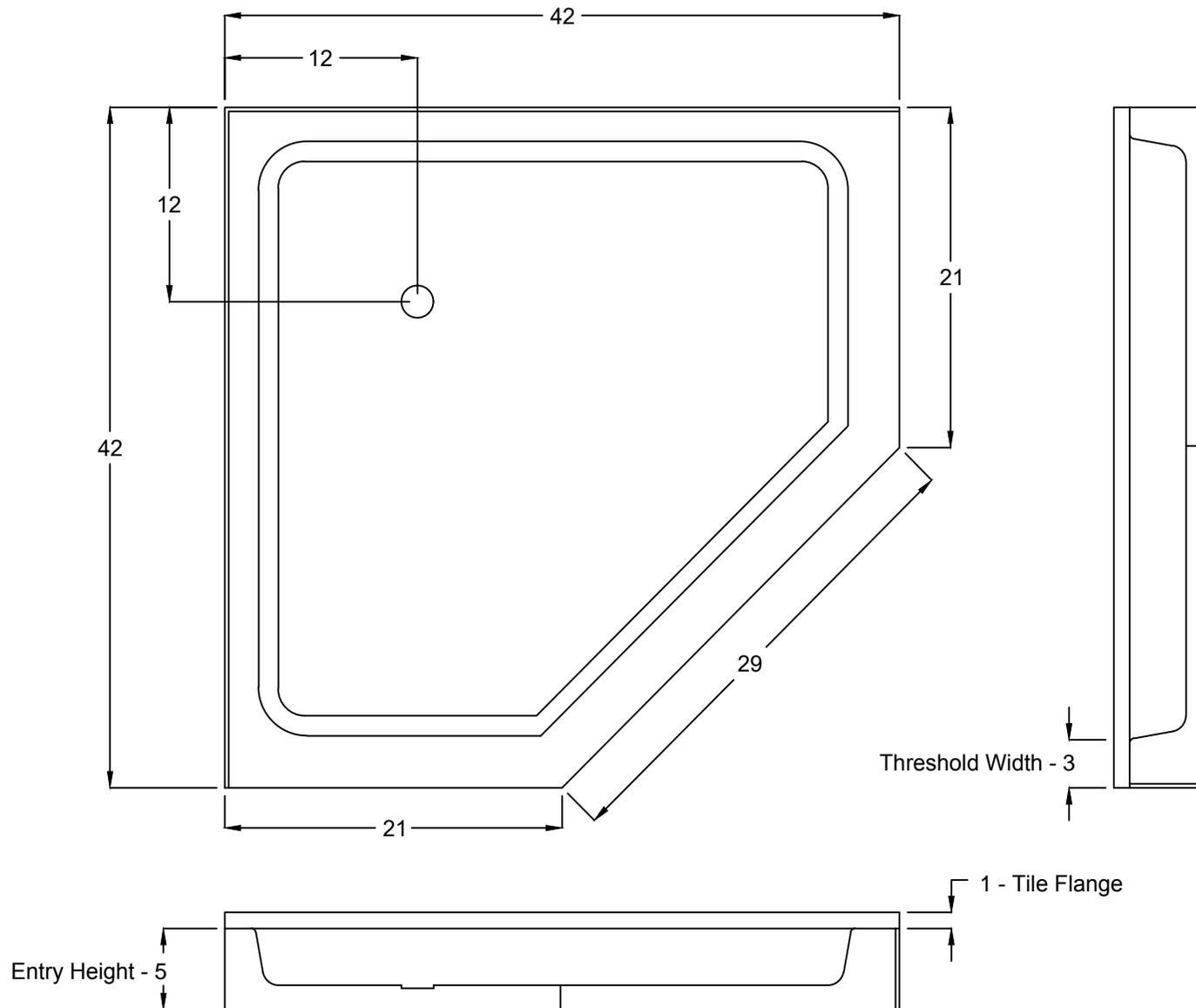
**Shower Pan Must Be Set in Mortar Base for Proper Installation**
