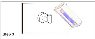
When the solid backing is in a pressed state, it's irradiated by a UV lamp with a certain intensity of light or sunlight. The irradiation principle is from the middle to the periphery, ensuring that the light can penetrate the bonding area and solidify the UV adhesive on the bonding surface.
