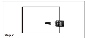
Use an appropriate amount of UV shadowless adhesive to the surface of the glass to be adhered, then close it with the solid backing to expel possible bubbles.
