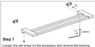
Loosen the set screw on the accessory and remove the backing plate. Position the accessory against the wall and mark outline with pencil.
