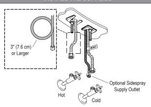
CAUTION: Risk of restricted water flow and product damage. Use extreme care to avoid kinking and twisting the supply hoses. The supply hoses must not be taut after installation.
